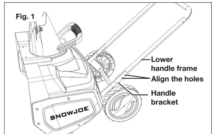
2. Secure the lower handle frame to the handle brackets with the 2 sets of knob and J-bolt, like shown (Fig. 2). Make sure the knobs are tightened.
